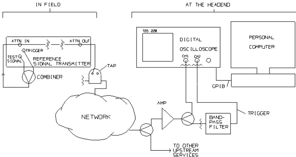
**Figure 1 Wiring Diagram for Measuring Upstream Frequency Response**
