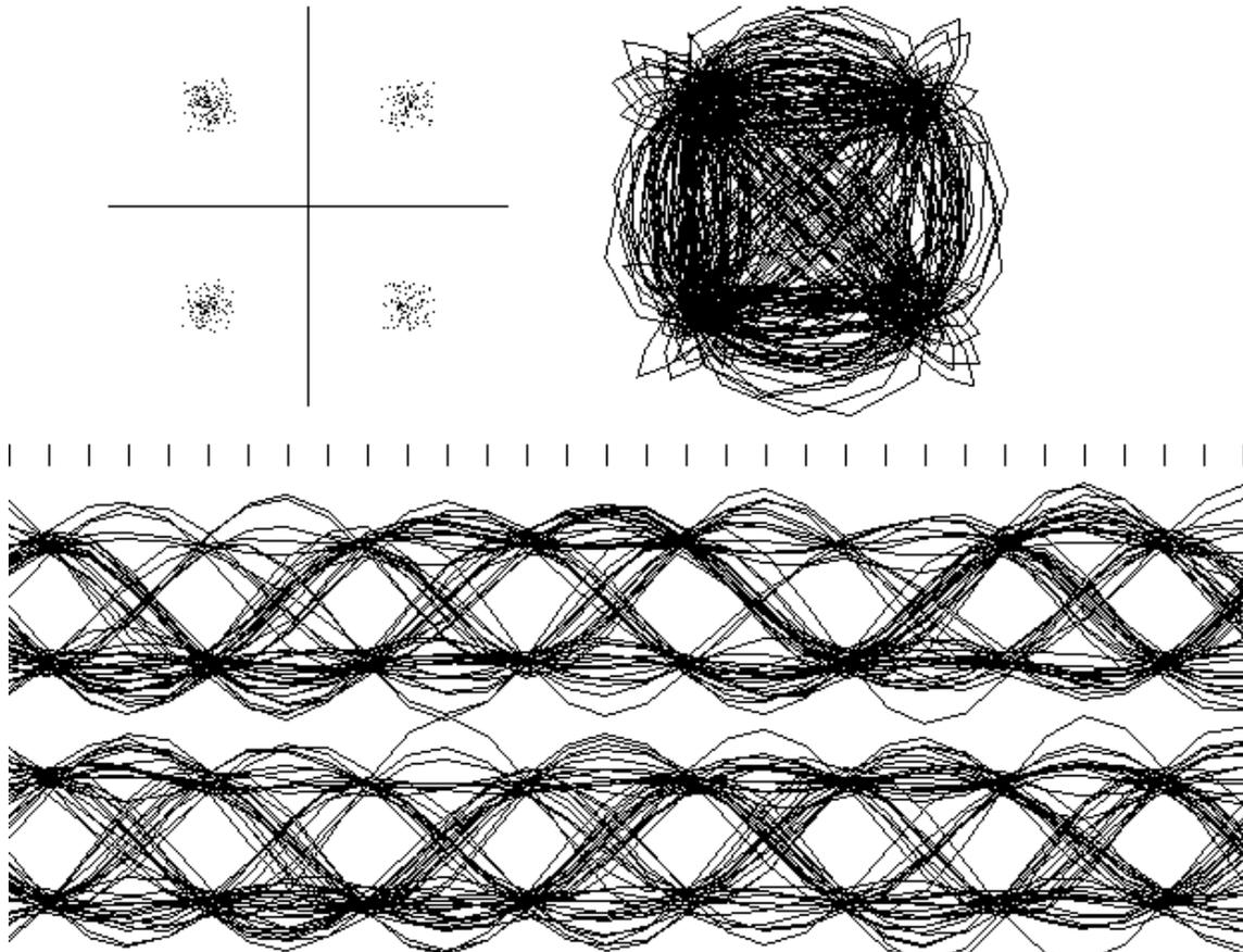
**Figure 8** A QPSK Constellation Plot and Eye Diagram of a Signal Distorted with 333 ns. of Group Delay Variation over 2.5 MHz. ; MER = 13.82 dB
