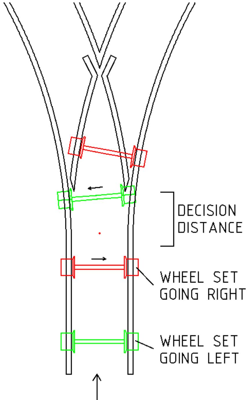
Figure 2. A junction illustrating a red rail wheel set going right and a green wheel set going left. Lateral force, shown as right and left arrows, determine which direction is taken by the wheel set at a junction. Force is applied over decision distance. There are multiple ways to apply lateral force.
