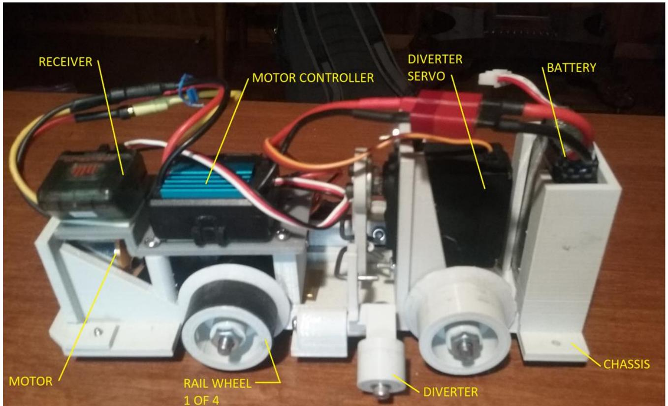
Figure 4. Side view of a model rail vehicle showing components. Not illustrated is worm gear transmission under motor controller.
