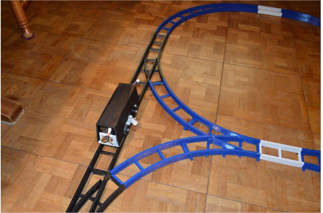
Figure 3. Model train on switchless tracks. Both vehicle and tracks were 3-D printed. The vehicle is made from PLA filament for precision. The tracks are made from ABS filament for strength.
